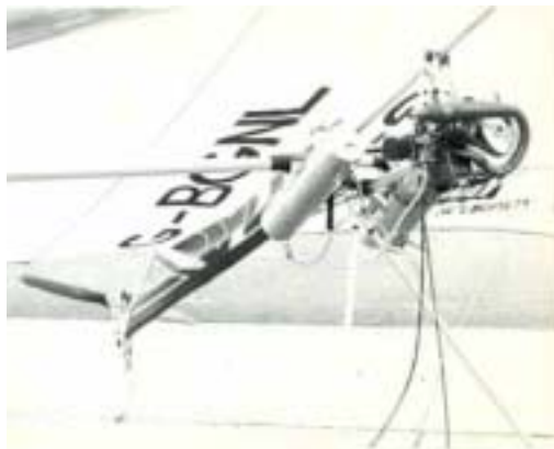
The Super Scorpion power unit and extra fuel tanks
